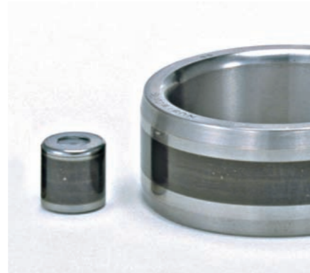
Fig. 4-2 Electric pitting generated on general purpose bearings (pits)
